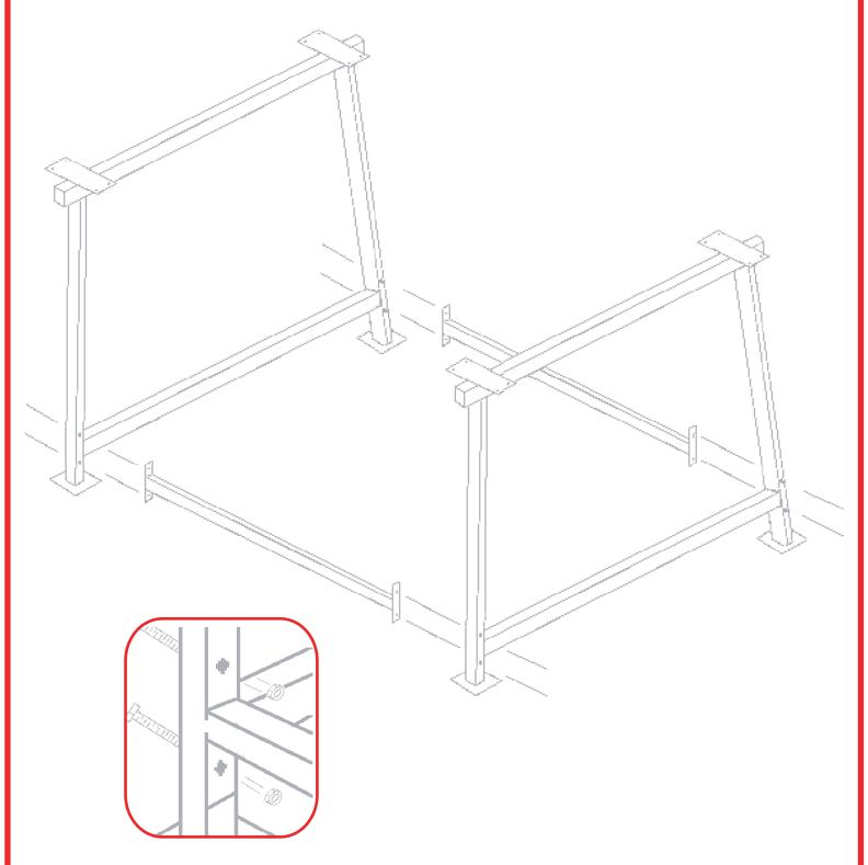
Fasten the two inch (2'') cross-members to the seven foot (7') main frames using eight (8) half inch by three and a half inch  $(1/2'' \times 3-1/2'')$  bolts, nuts, and locks.
