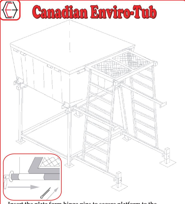
Insert the plate form hinge pins to secure platform to the Enviro-Tub. Making sure to insert the safety pins.
