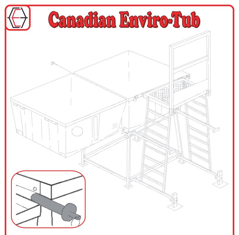
Connect the upper tub section to the lower tub section using two (2) hinge pins.
