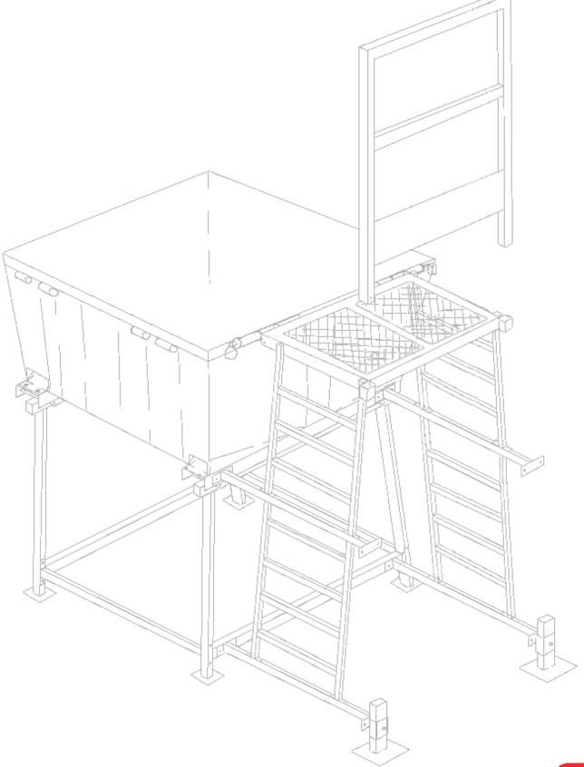
Insert the handrail into the platform handrail mount pockets and secure using two (2) safety pins.
