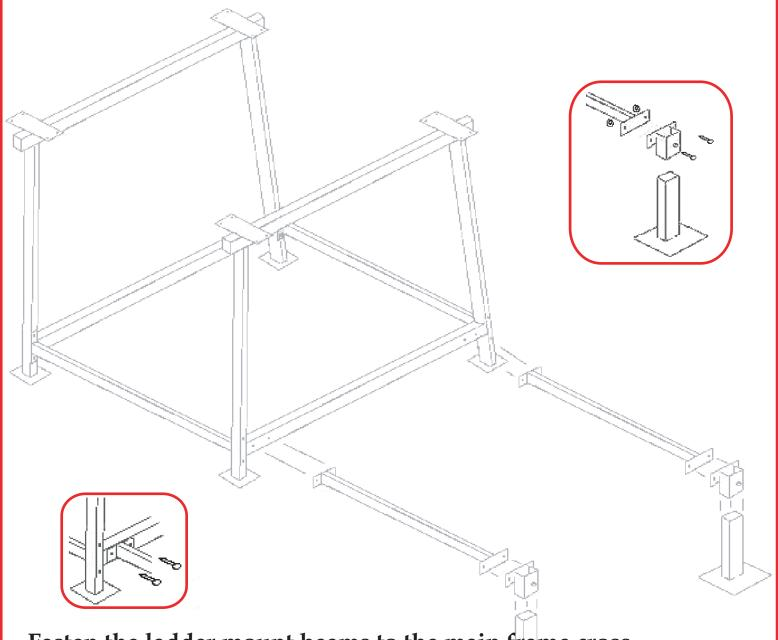
Fasten the ladder mount beams to the main frame cross beam using four (4) half inch by three and a half inch  $(1/2'' \times 3-1/2'')$  bolts, nuts and locks.
