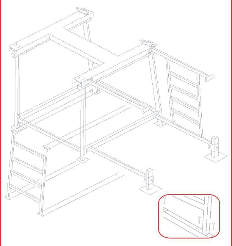
Fasten the bottom of the lower ladder sections to the ladder mount beams using eight (8) three-eights of an inch by two and a half inch  $(3/8" \times 2-1/2")$  bolts, nuts and locks.
