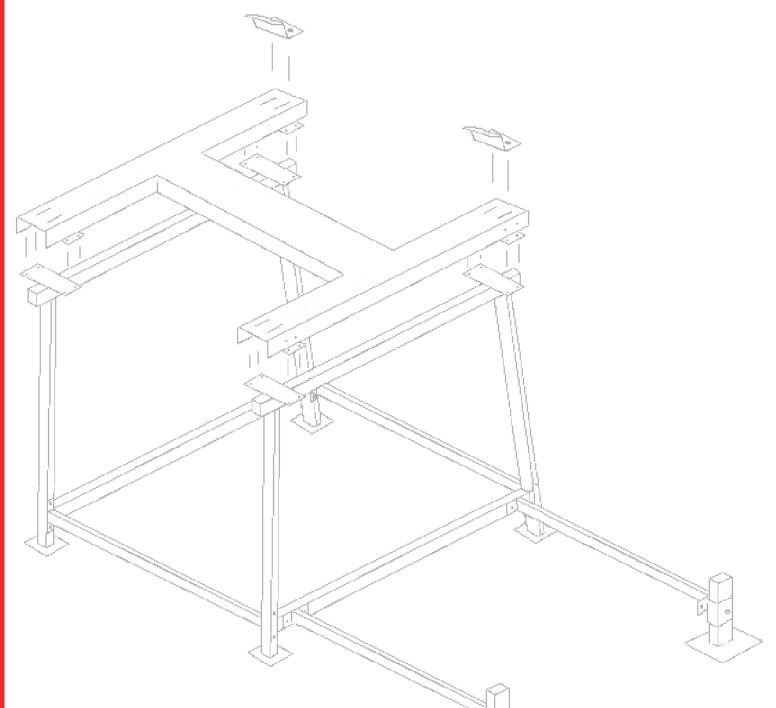
Mount the channel base frame to the main structure using sixteen (16) half inch by one and a half inch  $(1/2" \times 1-1/2")$  bolts, nuts and locks.
