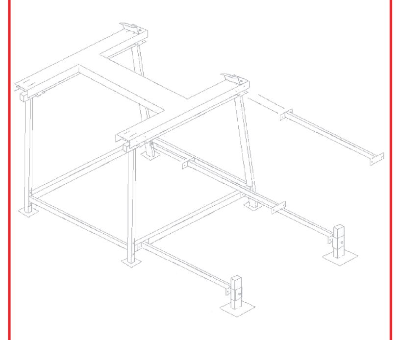
Fasten the intermediate ladder beams to the channel frame using four (4) half inch by one and a half inch  $(1/2" \times 1-1/2")$  bolts, nuts and locks.
