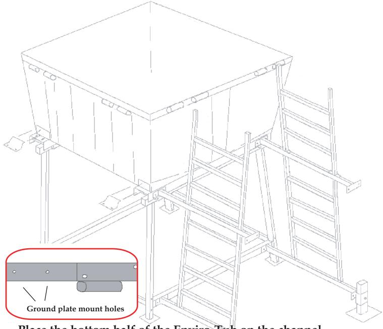
Place the bottom half of the Enviro-Tub on the channel frame.
