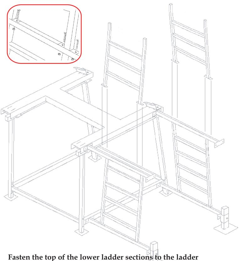
Fasten the top of the lower ladder sections to the ladder mount beams and upper ladder sections using eight (8) three-eights of an inch by three inch (3/8" x 3") bolts, nuts and locks.
